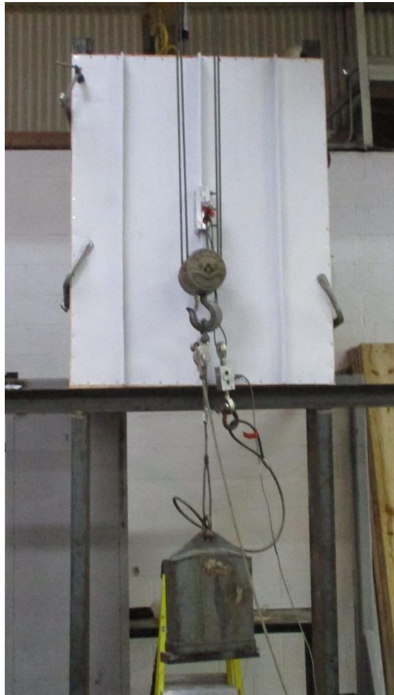
Photo No. 5 Dynamic Strength and Residual Strength Setup for Test Perpendicular to Direction of Standing Seam Roof
