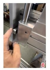
The bending arm can be fixed with the hook (6) on the left side of the machine.
